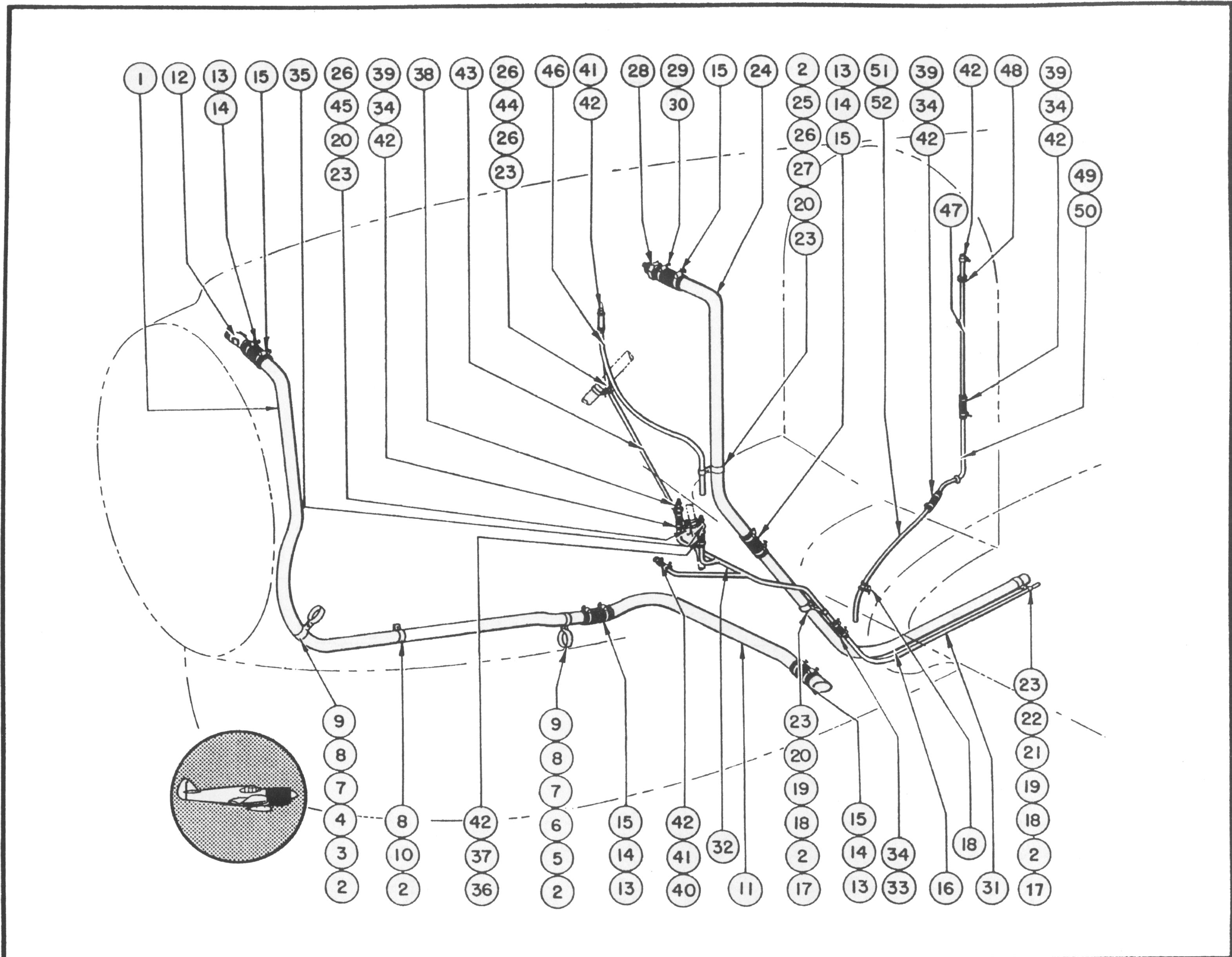
Figure 80—Breather and Vent Installation (C-W)
