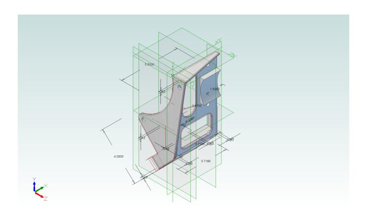
Support - Auxiliary Fuel Pump And Strainer - Cut view
